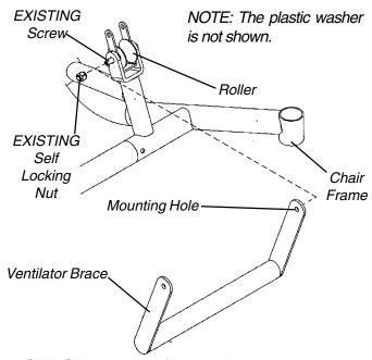
NOTE: Only one side of the ventilator brace attachment shown for clarity.
